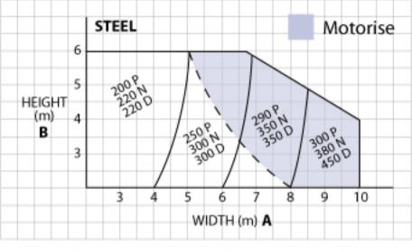
P = Pulley Headroom - min 430 for motorised N = Room Width - add 25 for motorised D = Room Depth
