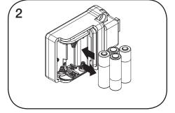
Remove the batteries from the housing. Replace with four premium alkaline AA batteries. Dispose or recycle used batteries according to local regulations.
